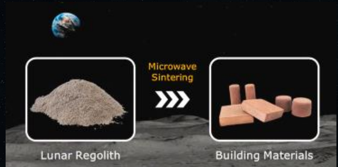
KLS-1 Lunar regolith simulant microwave sintered. Y.-J. Kim et al. Ceramics International, 2021
